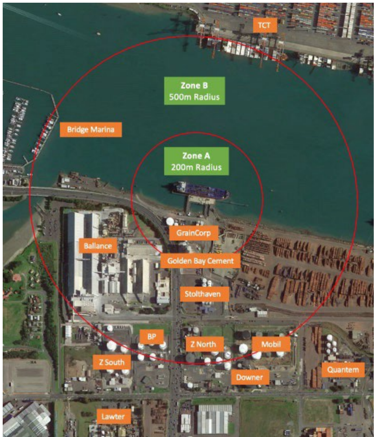
Figure 2: Tanker Berth – Evacuation Zones
