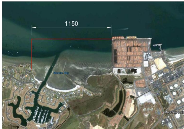
Figure 7: Potential Northport expansion required to replace the Port of Auckland's current and consented container terminal berthage
